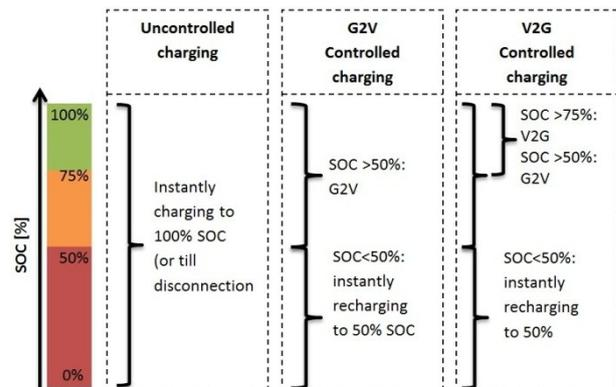
**Figure 3 – Example SOC levels for controlled G2V and V2G charging**
