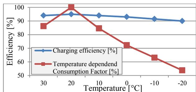
**Figure 2 – Example for temperature dependency of consumption and charging efficiency**
