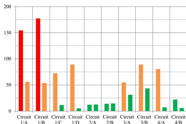
**Figure 9:** Comparison of the calculated results of the circulating currents in A for the original (left side) and optimized (right side) transposition, extension state II
