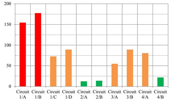
**Figure 6:** Calculation results of the circulating currents in A, extension state II
