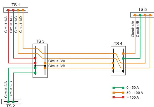
**Figure 5:** Illustration of the analyzed transmission line area, extension state no. II, with higher transport potential
