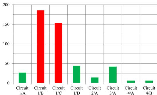
**Figure 4:** Calculation results of the circulating currents in A, extension state I
