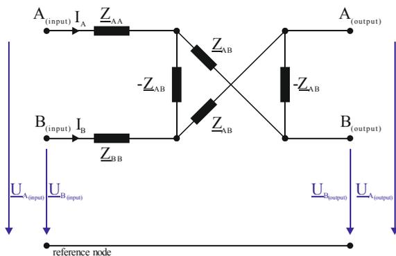
**Figure 2:** Applied mathematical equivalent circuit of two coupled phases (phase-to-earth loops) according to E. Clarke [5]
