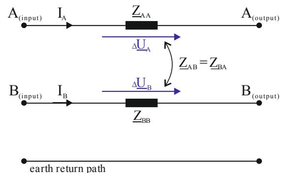
**Figure 1:** Fundamental illustration of two inductively coupled phases;  $\underline{Z}_{AA}$ ,  $\underline{Z}_{BB}$ ... self-impedance;  $\underline{Z}_{AB}$ ,  $\underline{Z}_{BA}$ ... mutual impedance;  $A_{(input)}$ ,  $A_{(output)}$ ... input and output nodes of the nodes auf the quadripole
