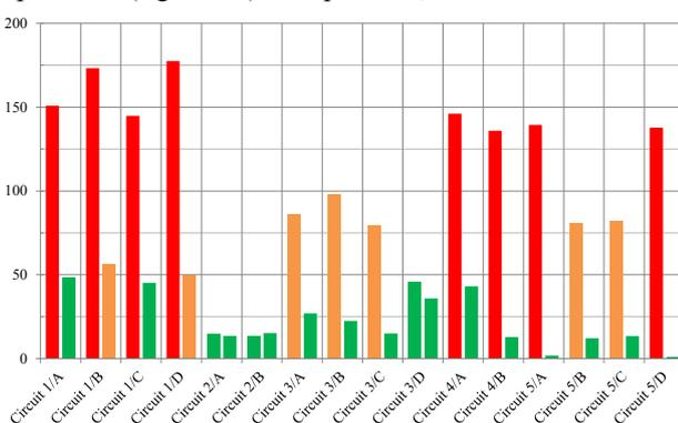
**Figure 10:** Comparison of the calculated results of the circulating currents in A for the original (left side) and optimized (right side) transposition, extension state III
